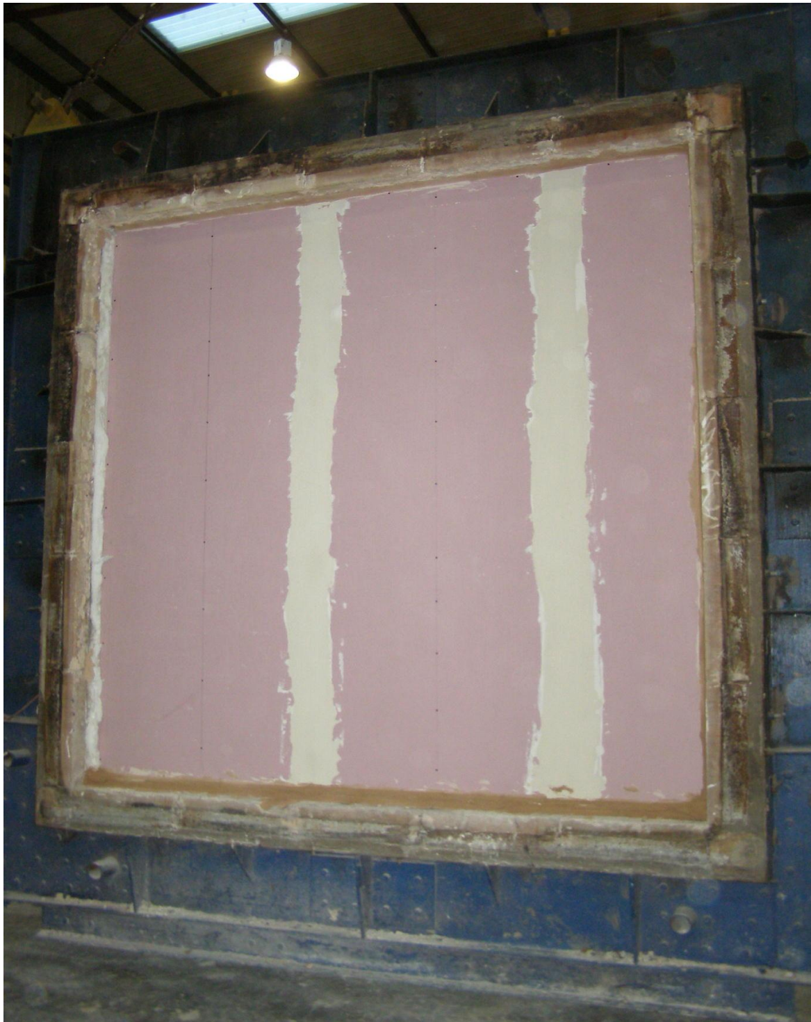
Photo 1 Exposed face of specimen before test.
