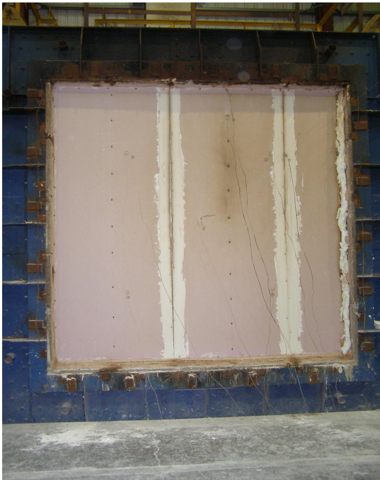
Photo 3 Unexposed face after 120 minutes.
