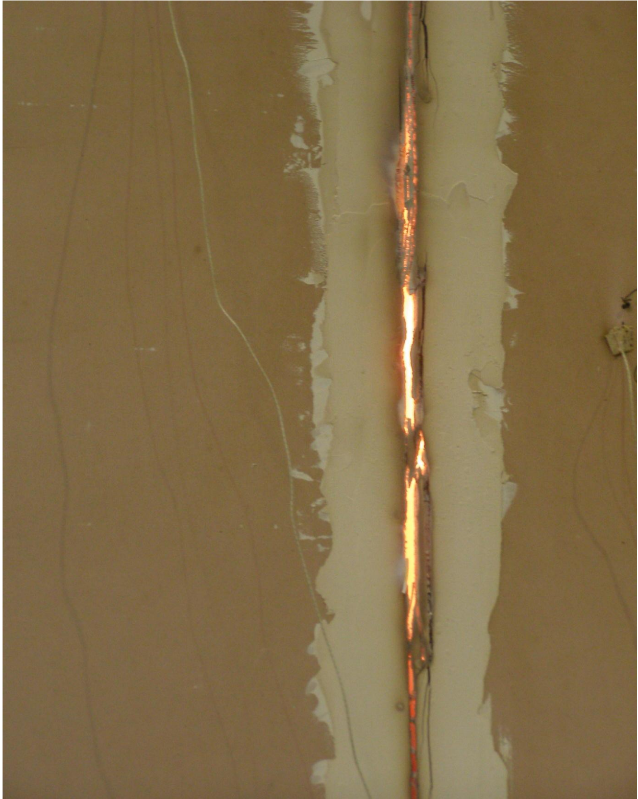
Photo 4 Location of integrity failure (129 minutes).
