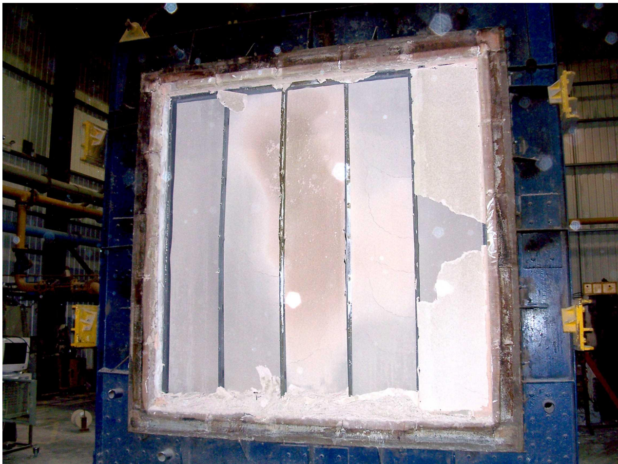
Photo 5 Exposed face of specimen after test.
