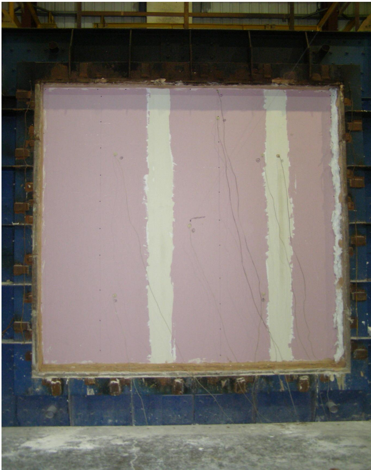
Photo 2 Unexposed face of specimen before test.
