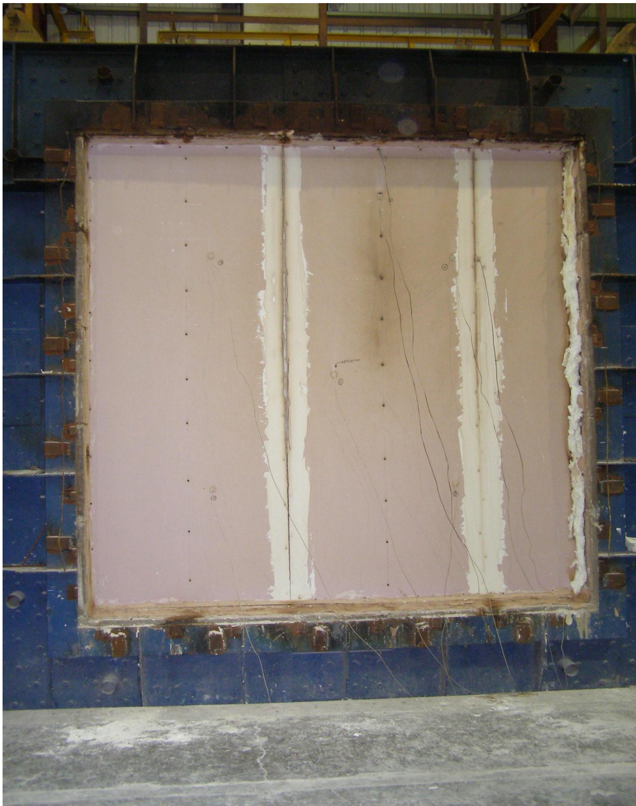
Photo 3 Unexposed face after 120 minutes.
